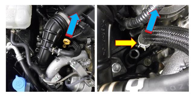
**3**. Fit the Forge silicone hose in replacement of the original turbo inlet hose. Using a 7mm socket and ratchet secure the hose using the supplied hose clamps. 40-60 clamp will secure the turbo end of the hose and the 60-80 hose clamp will secure the airbox end of the hose.
