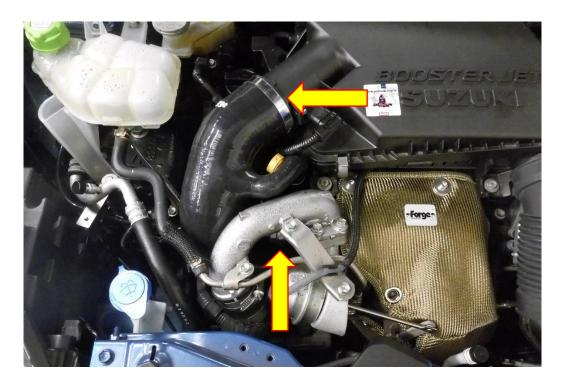
4. Using a 7mm spanner secure the oil breather hose to the engine using the 12-22mm hose clamp, then put the oil dip stick back in.
