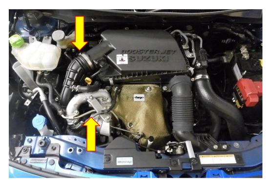
Pull out the engine oil dip stick and using some long nose pliers or hose removal tool loosen the hose clamp attaching the oil breather and remove the hose from the engine. The OE inlet hose can now be removed from the engine.
