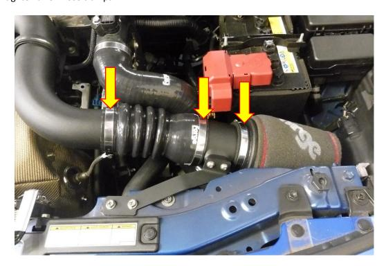
**18**. That is the installation of FMINDK53 complete, perform a spanner check in all areas which have been worked on then take the vehicle for a test drive and enjoy your new Forge Motorsport product.
