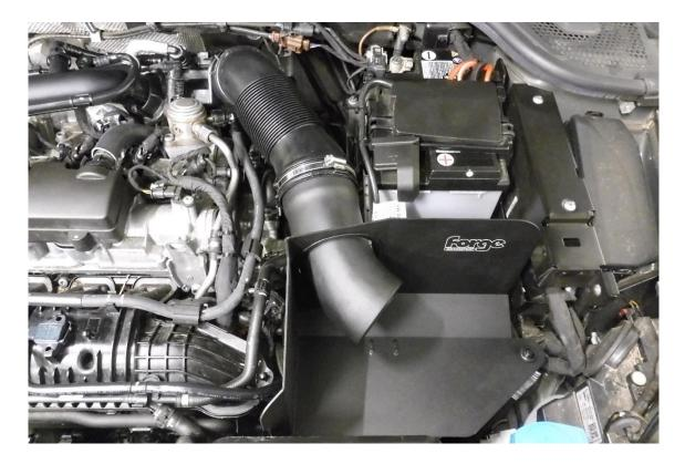
8. Fit the filter to the alloy pipe, adjust the angle of the pipe and filter until satisfied with its position, then using a 7mm socket and ratchet tighten both hose clamps and secure both the pipe and filter.
