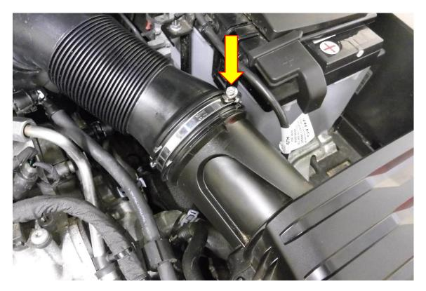
3. Pull the airbox sharply upwards to release it from its mounting points, then remove the airbox from the engine bay.
