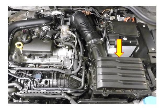
2. Using a 7mm socket and ratchet loosen the hose clamp attaching the inlet hose to the airbox, once loose detach it from the airbox
