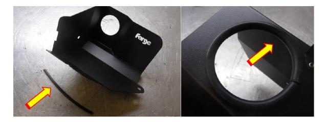
6. Place the Forge Motorsport air filter tray into position, angle it into the original air duct first then line up the rubber mounting points before pushing it firmly into place.
