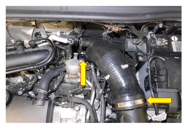
8. Take the breather adaptor and insert the billet end into the spout coming from the Forge intake hose. Secure it in place with the supplied 16-27 hose clamp.
