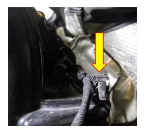
3. Using a T30 Torx drive loosen off the X2 fasteners attaching the turbo adaptor to the turbo.
