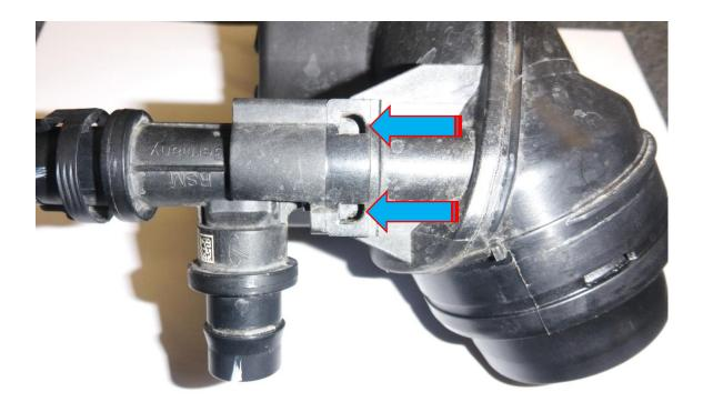
5. With the breather adaptor now removed, take the Forge Motorsport billet breather adaptor, and push it onto the end of the breather adaptor with the green O ring. There is a location marker on the billet adaptor which must be lined up with the plastic moulded line as shown in the picture below. Use the U clip supplied to secure the billet adaptor in place.
