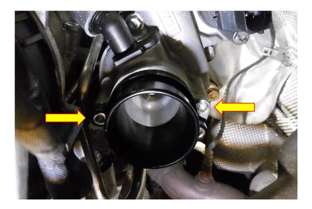
7. Fit the Forge silicone intake hose to the turbo adaptor, using a 7mm socket and ratchet or a flat bladed screwdriver fit the 50-70 hose clamp to secure it to the machined turbo adaptor and the 100-120 hose clamp to the air box.
