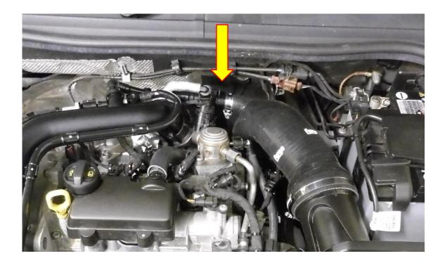
9. Connect both breather pipes back on to the breather adapter.
