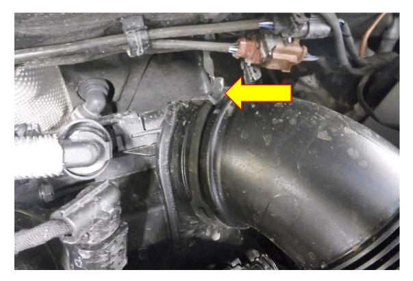
3. Fit the Forge Motorsport silicone hose in place large end to the airbox, small end to the turbo adaptor. Using a 7mm socket and ratchet secure the Forge Motorsport hose in place using the supplied hose clamps.
