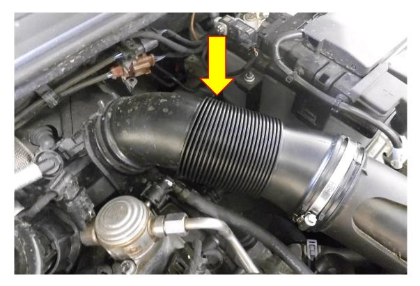
2. Using pliers or a hose clamp removal tool loosen the hose clamp attaching the inlet pipe to the turbo adaptor. The inlet pipe can now be removed from the engine.
