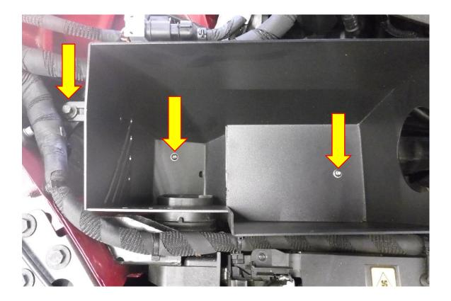
9. Using a 4mm Allen key remove the X2 fasteners attaching the MAF housing to the airbox lid, the MAF can now be removed.
