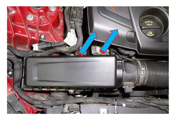
5. Using a 10mm socket and ratchet, remove the fastener attaching the lower half of the airbox to the vehicle.
