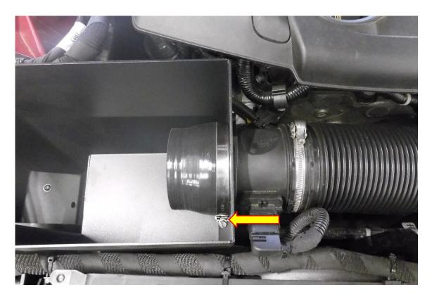
12. Take the alloy hose joiner and Forge air filter from the FMINDK49 kit. Push the alloy hose joiner to the dead stop in the neck of the Forge air filter. Using an 8mm socket and ratchet secure using the supplied hose clamp.
