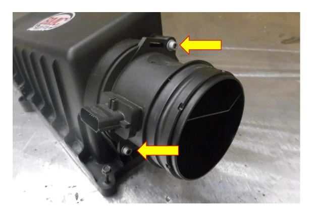
**10**. Re install the MAF housing to the inlet pipe and into the Forge airbox, reconnect the MAF wiring loom.
