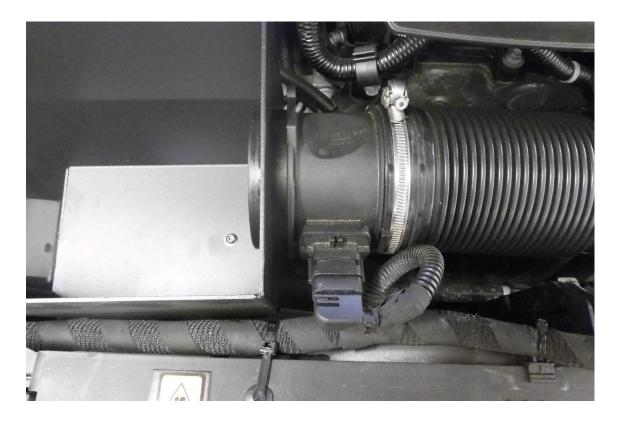
Take the silicone reducer hose from the FMINDK49 kit and attach the larger end to the MAF housing, using a 7mm socket and ratchet secure the hose using the supplied 80-100mm hose clamp.
