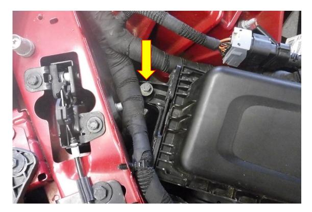
6. Pull the lower half of the airbox upwards off its rubber mounting points and remove it from the vehicle, this can be tricky so take your time.
