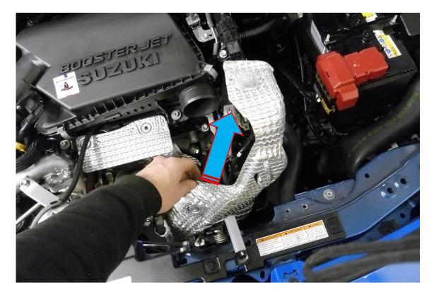
10. Place the FMTUBL19 into position while threading the lambda wiring loom through the large hole in the turbo blanket. Using a 5mm Allen key secure FMTUBL19 to the same mounting points as before using the supplied M6 fasteners and washers.
