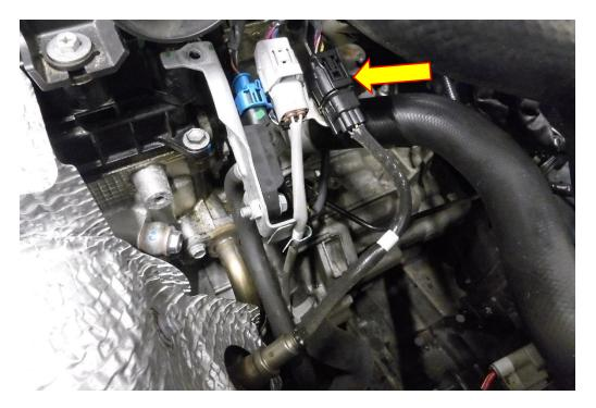
4. Using a 10mm socket and suitable drive, remove the X2 M6 fasteners holding the small upper OEM heat shield in place. DO NOT REMOVE THIS HEAT SHEILD.
