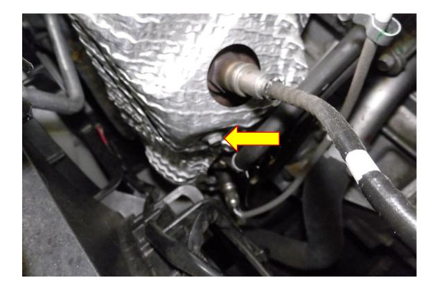
6. Using a Phillips screwdriver head and 10mm socket and suitable drive remove the fasteners attaching the undertray to the vehicle. Now remove the under try completely.
