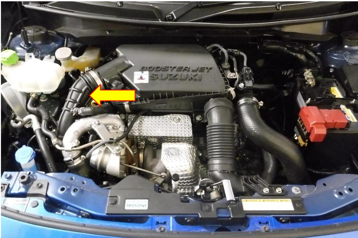
2. Using an 8mm socket and suitable drive or flat blade screwdriver loosen both hose clamps attaching the turbo inlet hose. Use plyers to loosen the hose clamp attaching the breather hose and disconnect it from the turbo inlet hose. You will now be able to remove the turbo inlet hose from the vehicle.
