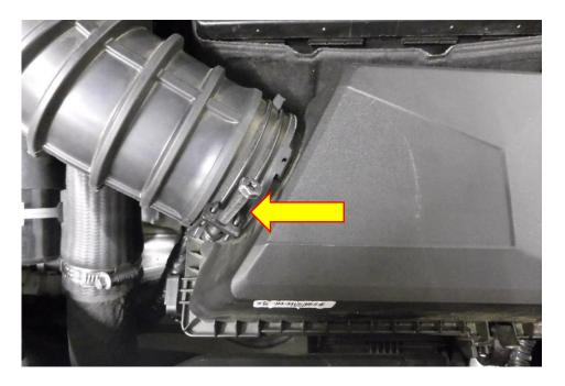
**3**. Using a 10mm socket and ratchet with extension remove the X3 M6 fasteners attaching the airbox to the vehicle.
