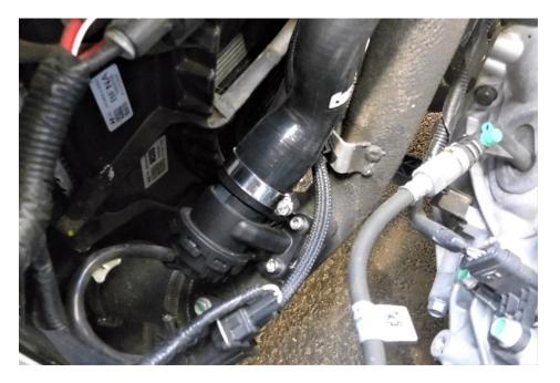
7. Follow steps 1-4 in reverse order, but now securing the other end of the Forge dump valve discharge hose to the inlet hose with the supplied 20-32mm hose clamp using a 7mm socket and ratchet.
