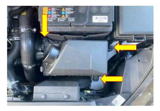
4. Using a flat bladed screwdriver prise the X2 plastic retaining clips open and remove them from the air duct to the airbox. You will now be able to remove the airbox from the engine bay.
