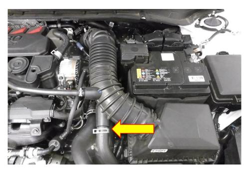
2. Using a 10mm socket and ratchet loosen the hose clamp attaching the inlet hose to the airbox, once loose detach the inlet hose from the airbox-
