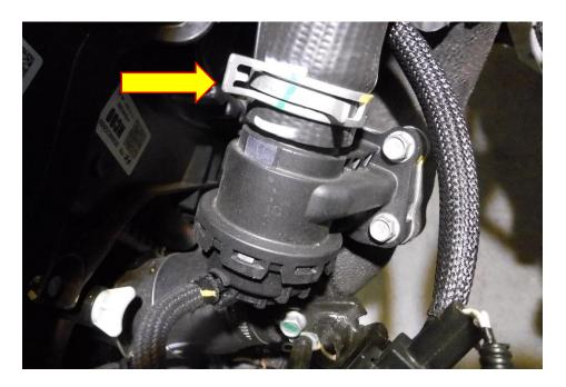
6. Fit the larger end of the Forge discharge hose to the valve and using a 7mm socket and rachet secure it using the 25-40mm hose clamp.
