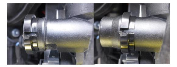
4. Push the supplied adapter over the pipe ensuring the slot is over the split sleeve
