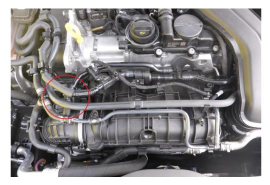
2. Squeeze the connector and disconnect.
