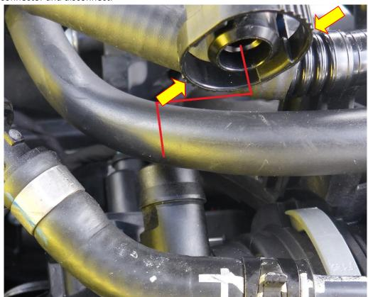
3. Take the supplied split sleeve and slide it over the taper on the pipe
