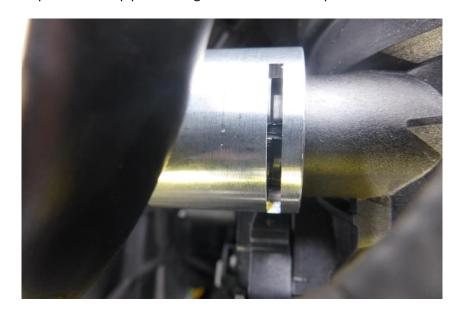
5. Fit the supplied horseshoe shaped clip and refit the vacuum connector.
