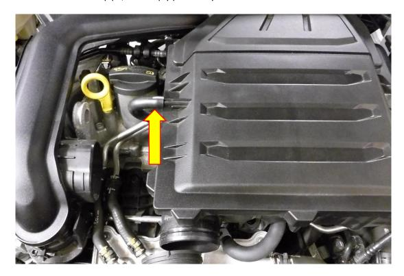
4. Now you will be able to remove the airbox from the engine bay, this should just pull out
