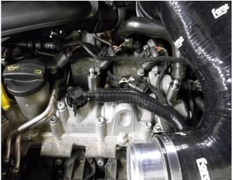
10. Using a trim removal tool or flat blade screwdriver remove the two rubber mounting grommets from the airbox, take your time as they are tightly fitted.
