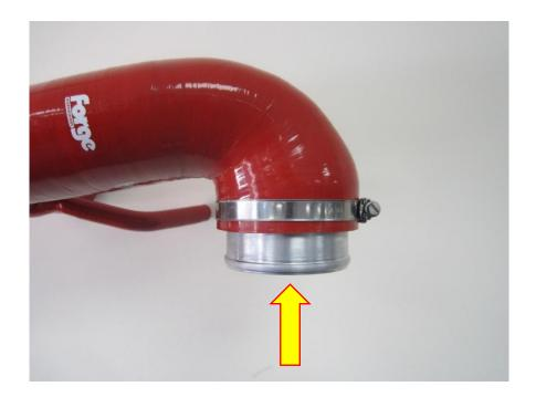
7. Fit the silicone hose at the joiner end to the OE rubber inlet hose and push it in so it's seated snugly. Again, you will need to use a spring clamp removal tool or pliers to secure the joiner to the OE rubber inlet hose. Attach the extended silicone hose to the oil breather as shown in the picture.
