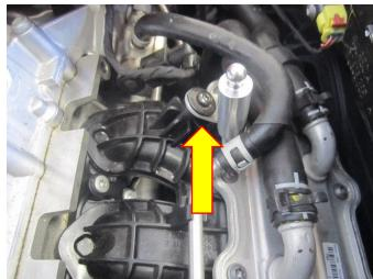
9. Using a 10mm spanner remove the original air box mounting pegs and replace them with X2 machined **SHORT** mounting pegs from the FMINDK39 kit on top of the rocker cover, these only need to be hand tight.
