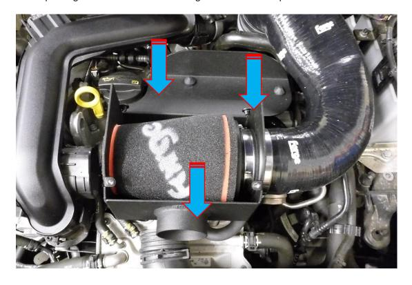
14. Re attach the air intake scoop to the front of the heat shield and using a 4mm Allen key attach the lid of the heat shield using the supplied M4 fasteners.
