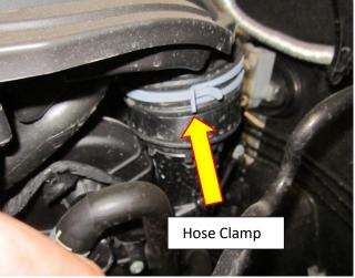
3. Remove the oil breather pipe, this simply pulls away from the airbox.
