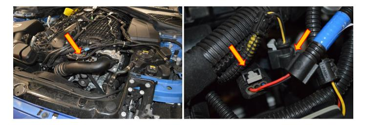
3. Using a T30 Torx drive, remove the 3 fasteners that hold the boost pipe flange to the throttle body.
