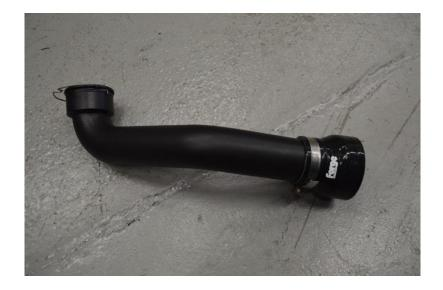
11. Fit the lower boost pipe and ensure the retaining clip is fitted fully and securely.
