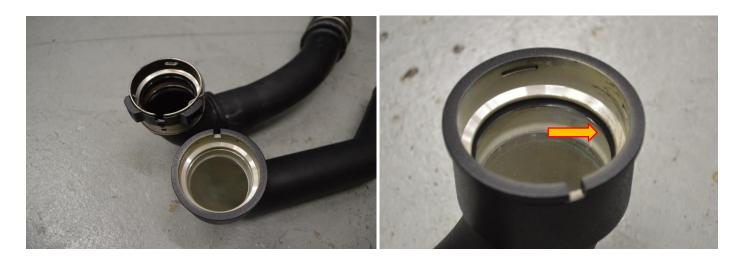
9. Using a T20 torx drive, remove the OEM map sensor from the plastic boost pipe, then remove the air temp sensor by unscrewing anti-clockwise. These can now be fitted into the new Forge alloy hard pipe using the fastener provided. If you are not using water meth, use the blanking plug provided and a 12mm spanner to block the meth injection port.
