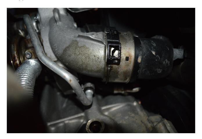
**6.** Using a flat headed screwdriver or pick, disconnect the retaining clip on the boost pipe coupler and remove from situ as pictured below.
