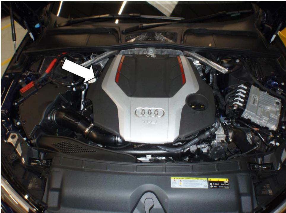
3. Disconnect the wiring to the standard dump valve. Using T30 Torx driver undo 3x bolts and remove the OEM dump valve.
