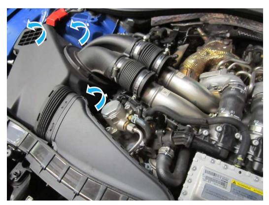
9. Using a 4mm allen key ensure the 4 allen caps that hold the performance airfilter into the carbon fibre airbox are tight.
