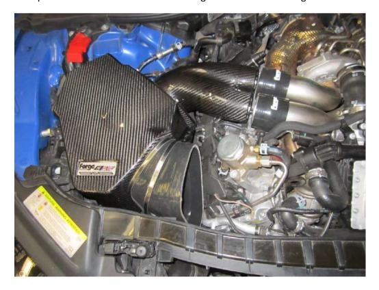
14. Slide the carbon fibre scoop fully into the triangle silicon hose, do not tighten any of the hose clamps at this stage.
