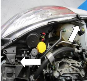
**13.** Now remove the 2 radiator clips and the 1 intercooler clip on the slam panel by turning them anti clockwise.
