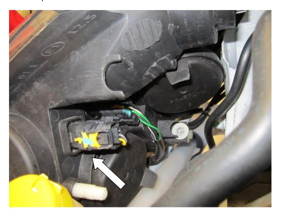
**12.** Now using a 10mm socket remove the 3 fasteners that hold the headlight in place, then remove the headlights.
