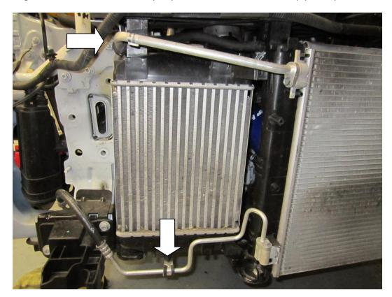
**15.** Now remove the two fasteners with your 13mm socket that hold the slam panel in place, then remove the slam panel.
