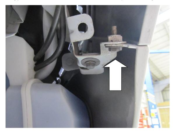
**7.** Disconnect the loom to the DRLs found inside the passenger wheel arch on RHD vehicles.
