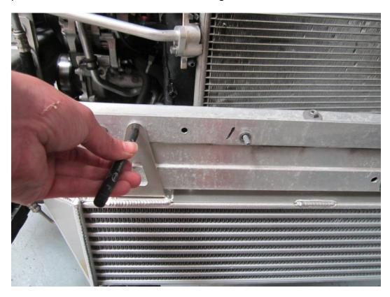
**23.** Now again using your 7mm drill bit drill the second hole then use another of the allen caps provided to mount into position. Use your 6mm allen key and 10mm spanner to tighten both of these fasteners.
