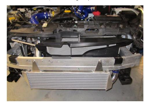
**29.** Using the bracket provided clamp the cowling into position by pushing the bracket downwards, and then tighten the nut with your 10mm socket.
