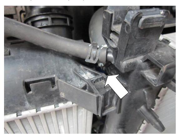
19. Now remove the intercooler, this lifts out of the sub frame and radiator mounts.
