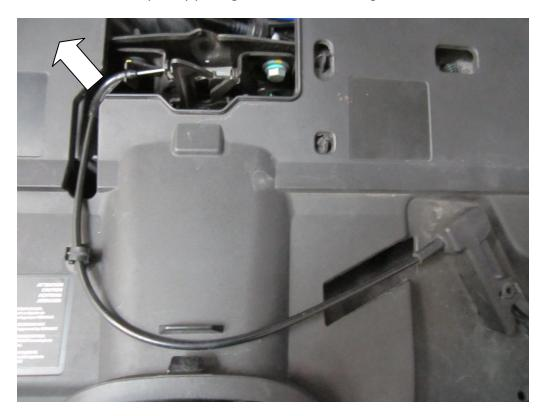
**6.** Using your 10mm socket remove the bolts that hold the bumper to front wings.
