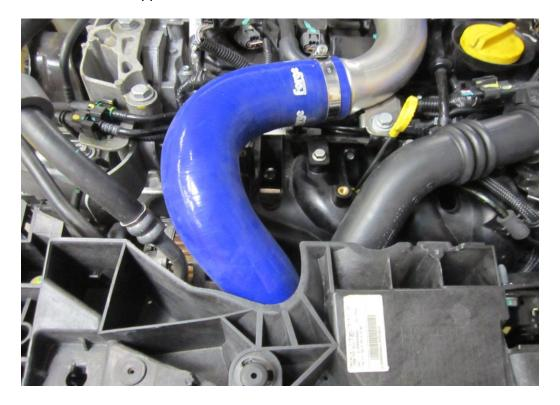
**25.** Now fit the p-clip around the hard pipe and mark your final hole to drill in the crash bar. Again use a 7mm drill bit then using your 6mm allen key and 10mm socket tighten into position .This p-clip must be fitted in order to stop the hard pipe rubbing the condensor.
