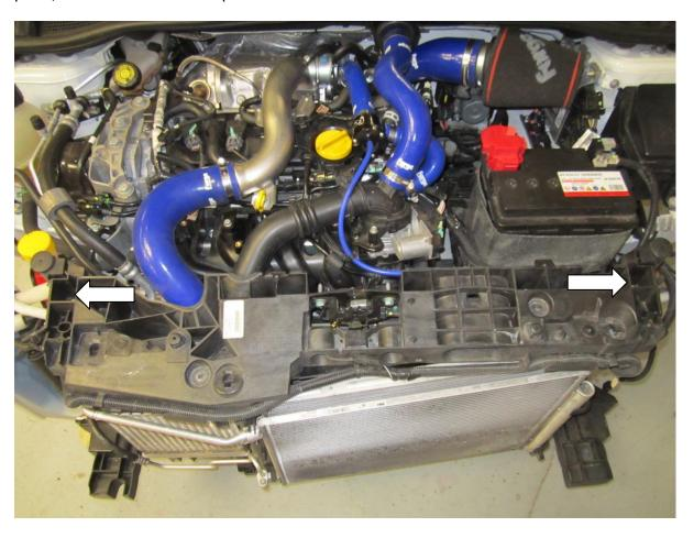
**16.** Now by pushing in the the clips on the condensorand pulling gently, remove the condensor from its locating points and slide towards the drivers side. Be careful not to damage the condensor or pipes.
