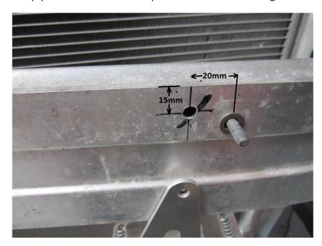
**22.** Now this is marked use a 7mm drill bit to drill the hole. Then place the 6mm Allen cap provided through the bracket and hole, and swing the intercooler up into position to mark a hole for the other mounting bracket .
