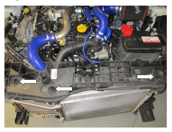
**14.** Using a 7mm socket remove the p clips that hold the condensor pipes in place.
