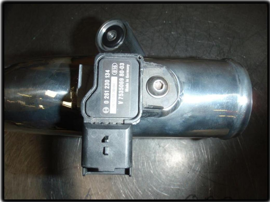
4. Fit the boost inlet pipe first as the bolt by the dip stick is hard to get too, use the bolts and washers supplied in the kit.
