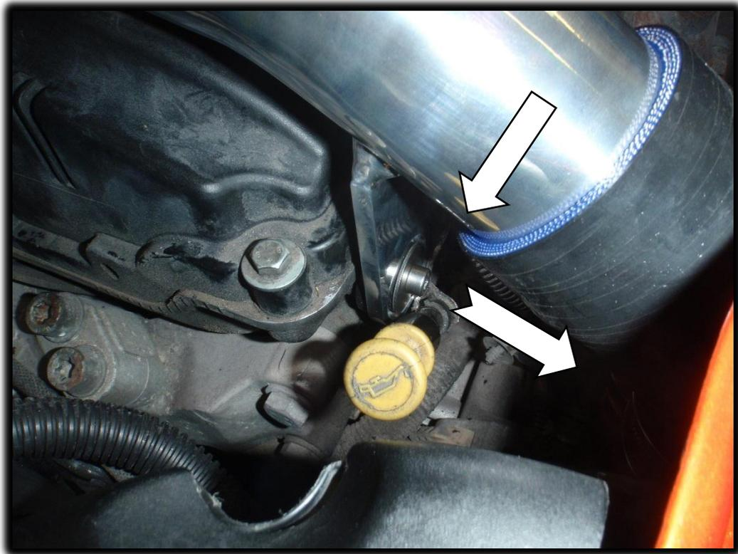
6. Once the inlet boost pipe is fitted and secured attach the boost outlet again using bolts and washers supplied.
