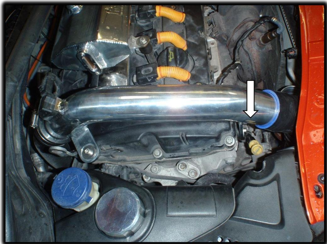
5. The fitting of the inlet boost pipe will be made easier if the dip stick and bracket is eased forward.
