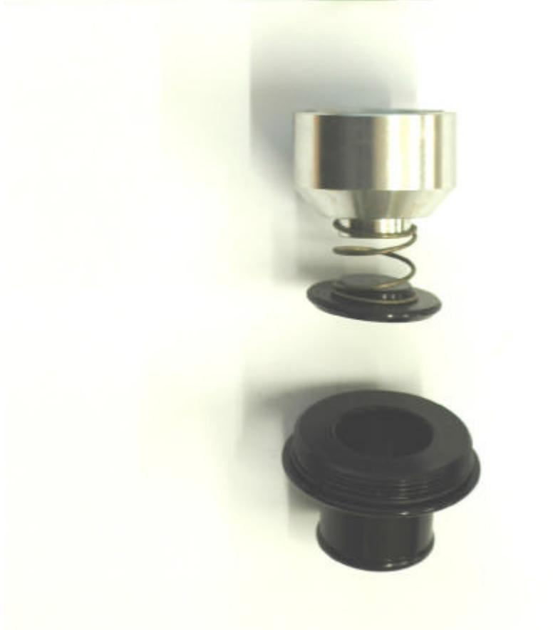
Assemble the spring top plate onto the spring. The smaller diameter end of the spring fits into a recess in the spring top plate.
