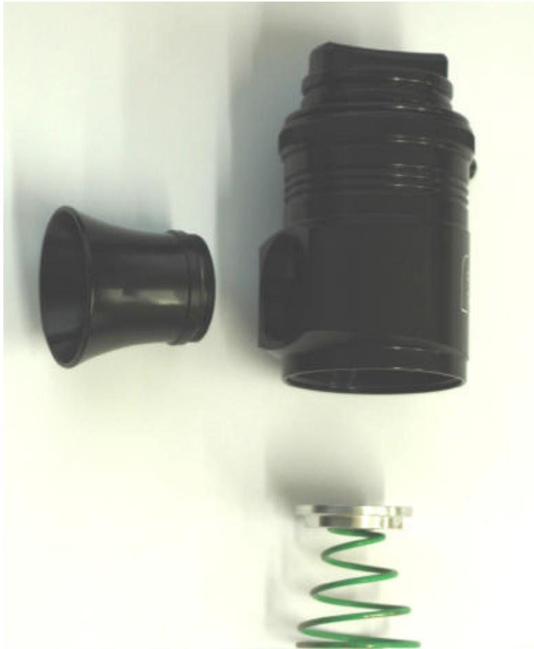
Screw the side bell mouth trumpet into the valve body
