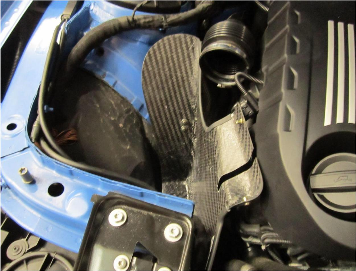
**16.** Remove the MAF sensor from the OEM plastic inlet pipe and fit into the carbon fibre inlet pipes with the fasteners provided.
