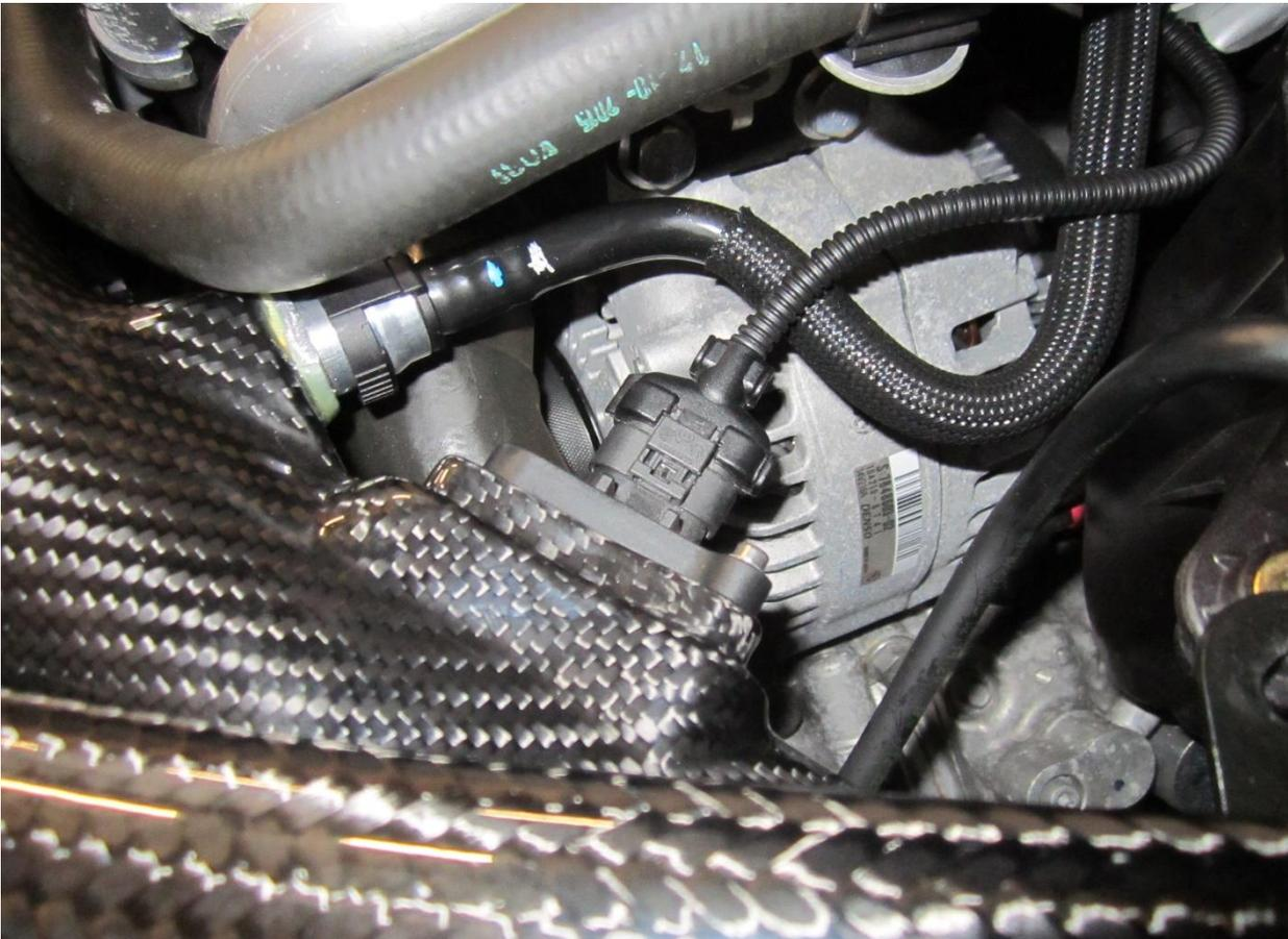
21. Ensure the wiring loom is connected to both MAF sensors.
