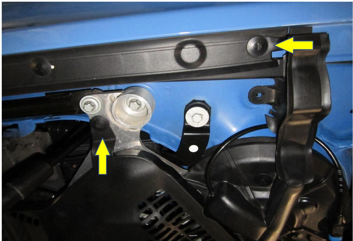
4. On both sides of the vehicle, use a 10mm socket to turn the fasteners 180 degrees to remove the plastic covers.
