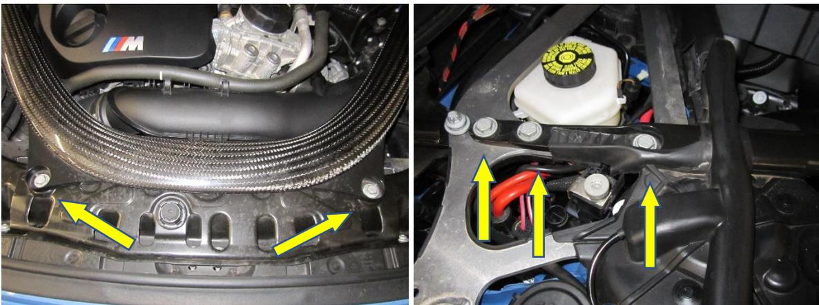
6. Undo the 10mm fastener that holds the charge cooler expansion tank to the strut brace.
