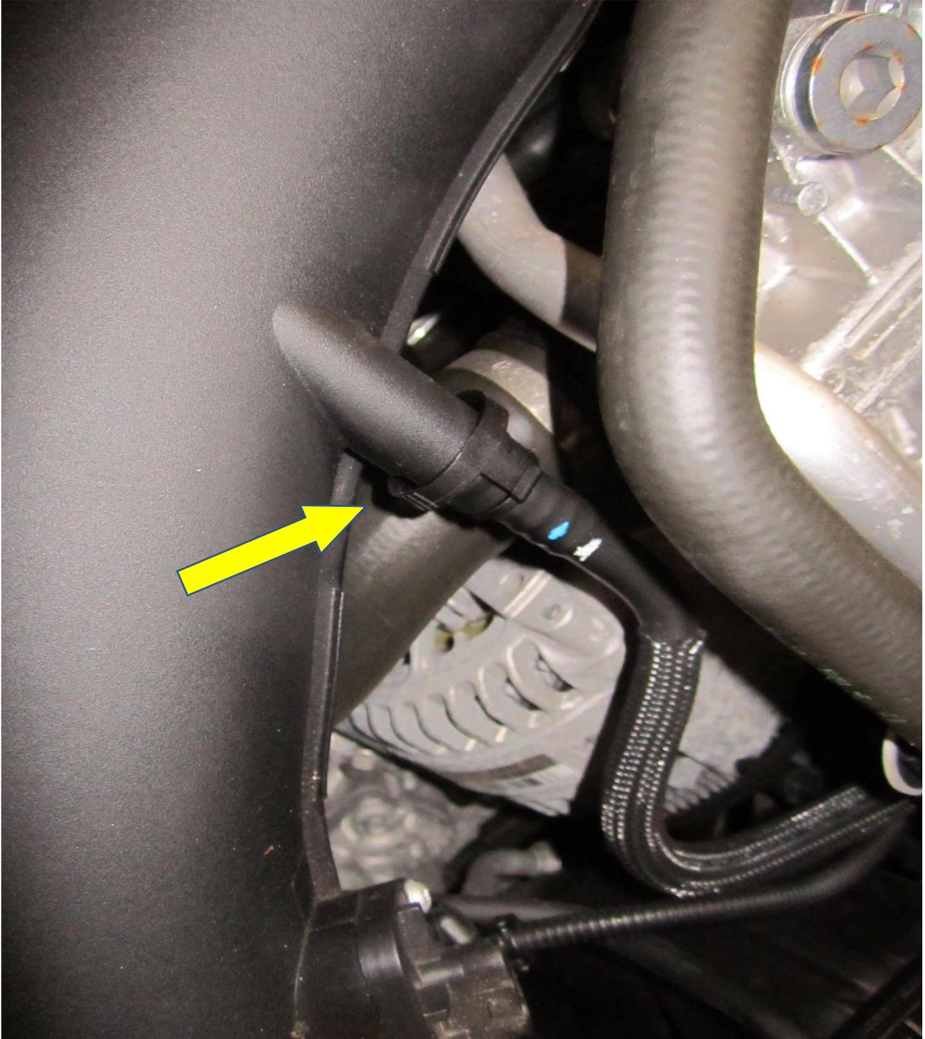
11. The longer inlet pipe can now be removed.
