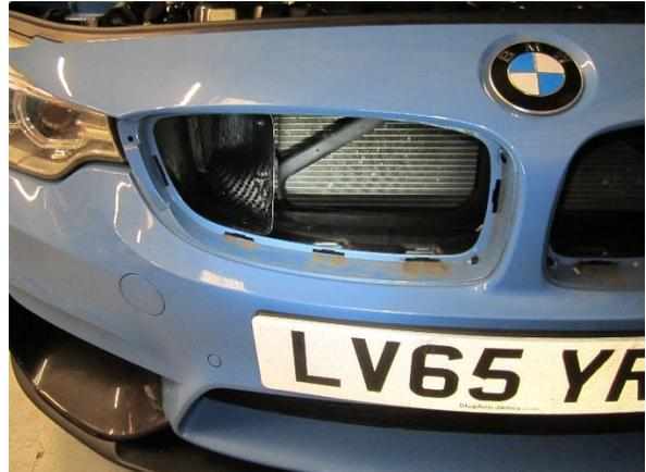
14. Remove the fastener arrowed below with an 8mm socket.
