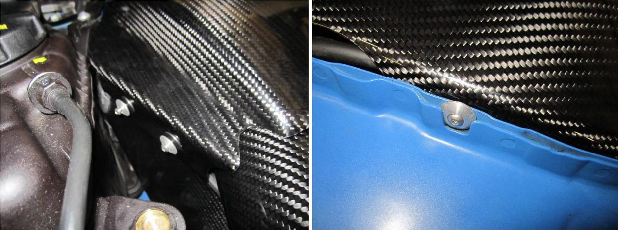
20. Re-attach the air breather to the longer carbon fibre intake pipe.
